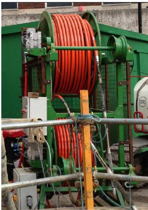
PICTURE 2: Tilt switch attached to a grout reel.
