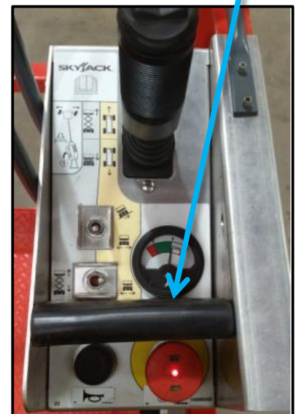
Sensor bar ergonomically situated in front of the joystick/controls
