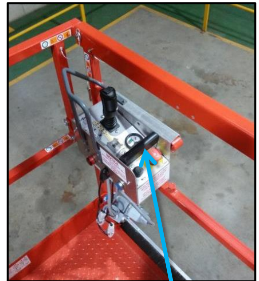
Sensor bar ergonomically situated in front of the joystick/controls
